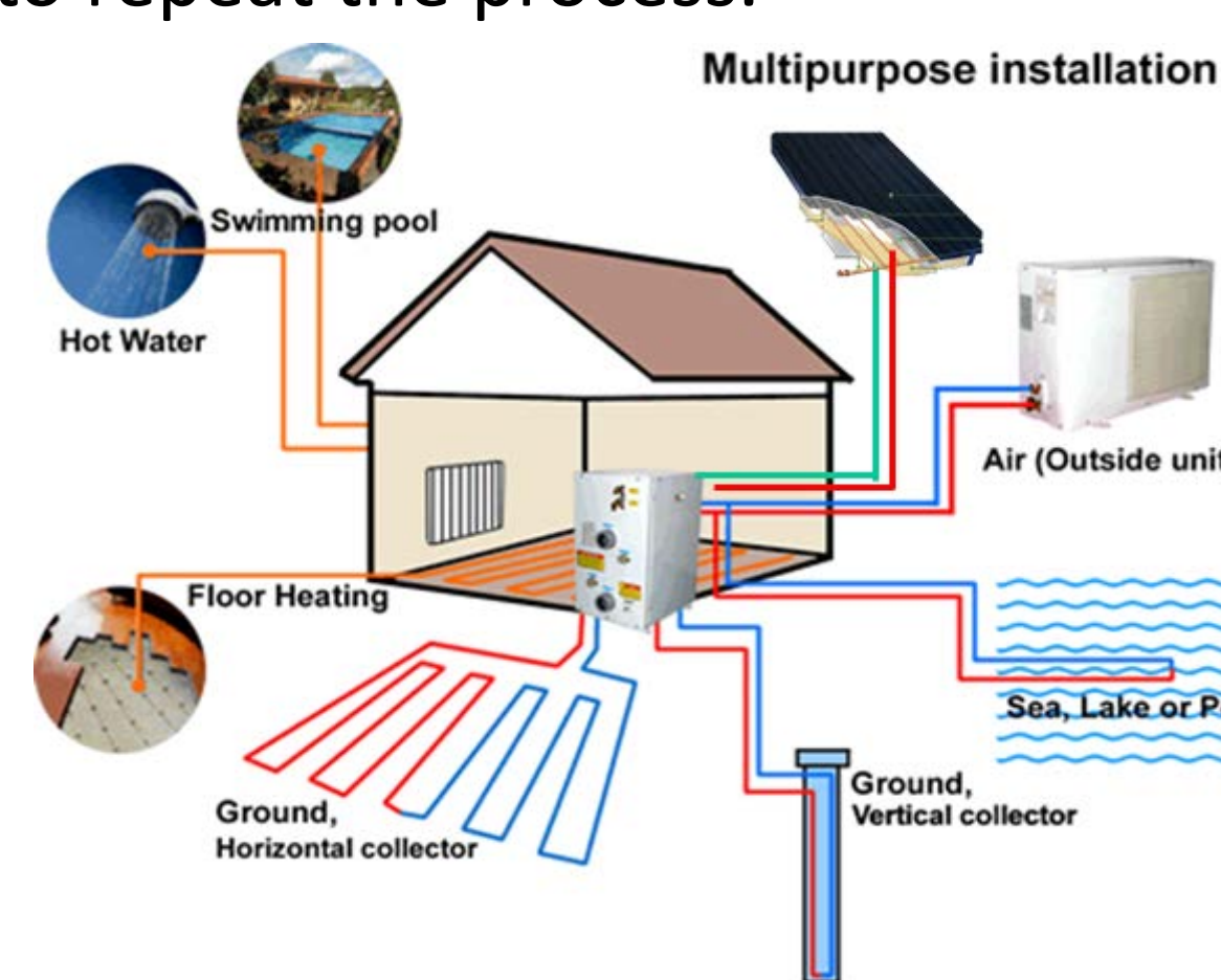
Figure 2: Sources of energy for heat pump system
