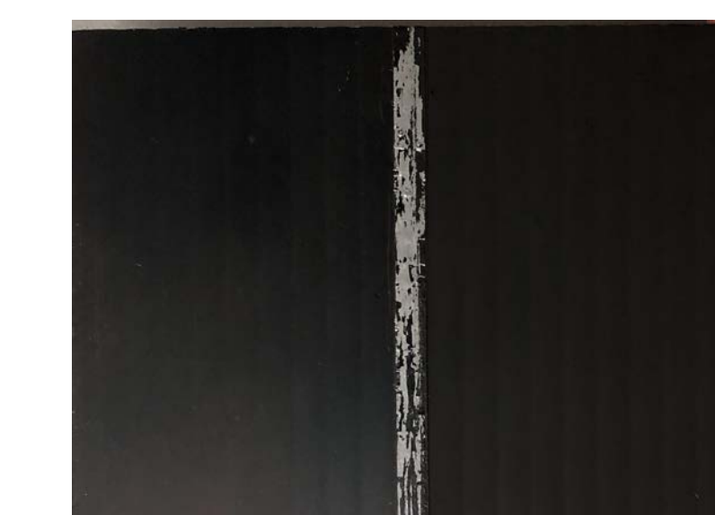
Figure 6: Test paint panel. Left side is flat black paint and right side is ThurmaloX Solar Collector Coating paint. ThurmaloX is designed to absorb more sunlight energy than ordinary flat black paint. It is specifically intended to be used with solar water heater collectors.
