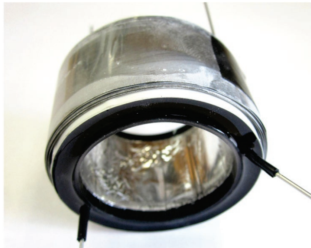
Figure 4-3 View of device 3 core with inductor windings removed to show concentric electric field and magnetic field core arrangement.
