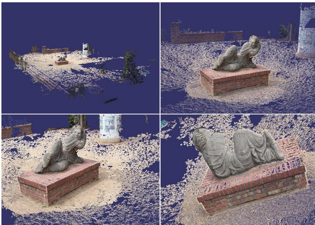
Figure 45 Dense Point Cloud Generation from Triangulated Points Der Hass
