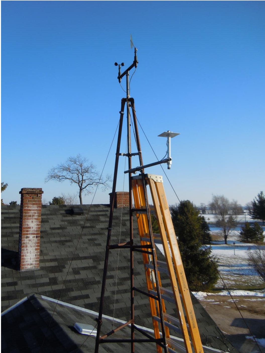
Fig. 10-7: Wind vane and solar radiation sensors on roof of house.
