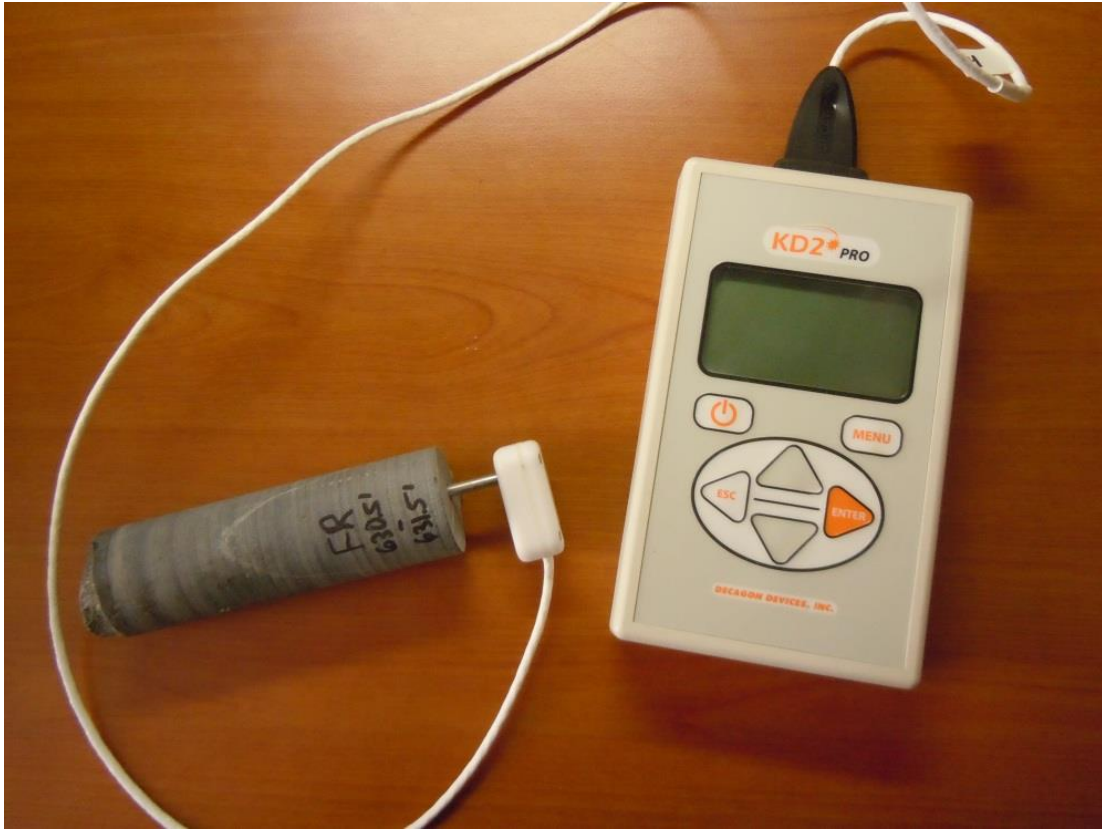
Fig. 9-1: KD2 Pro set up with the RK-1 probe in Sample FR (Precambrian Andesite).
