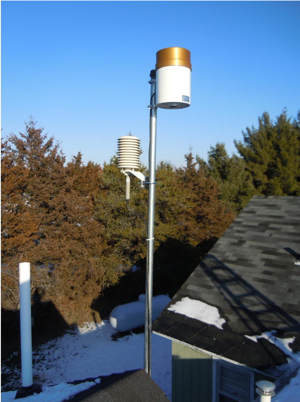
Fig. 10-8: Tipping bucket, relative humidity and temperature sensors on roof of house.
