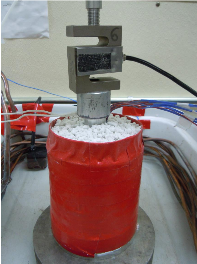
Fig. 3-3: Close-up of testing cell with applied load.
