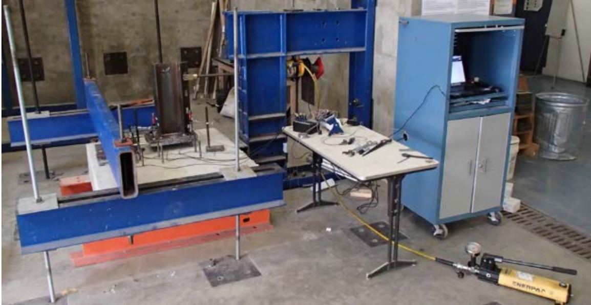
Figure 2.33 Eccentric Shear test setup
