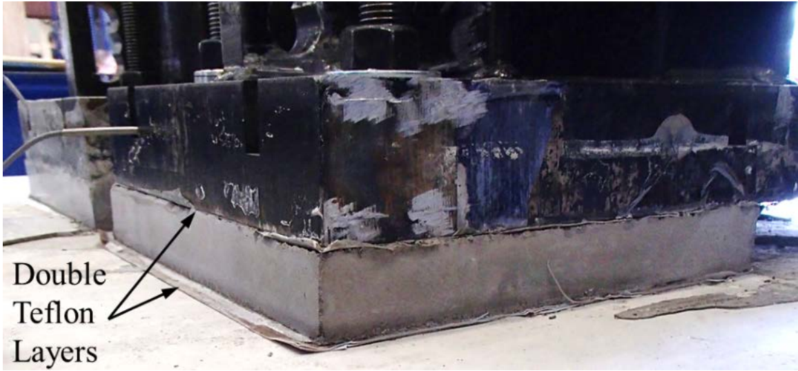
Figure 2.39 Eccentric shear test setup by McBride et al. (2014).
