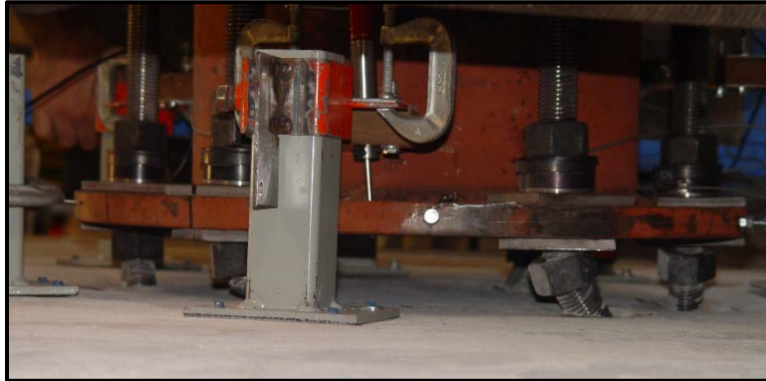
Figure 2.31 FS1 anchor bolts in failed condition
