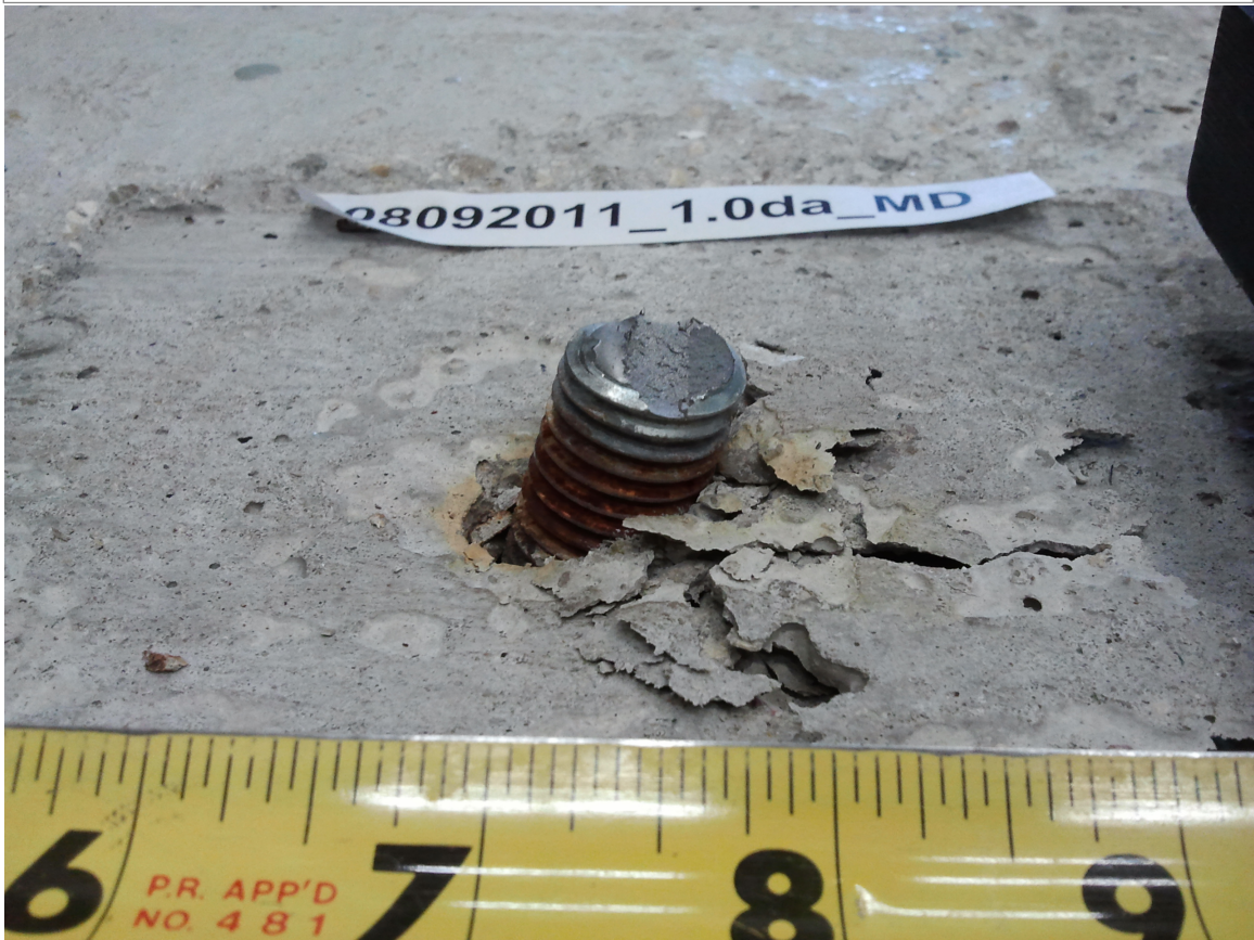
Figure I.12 Behavior of Specimen 08092011_1.0da-MD
