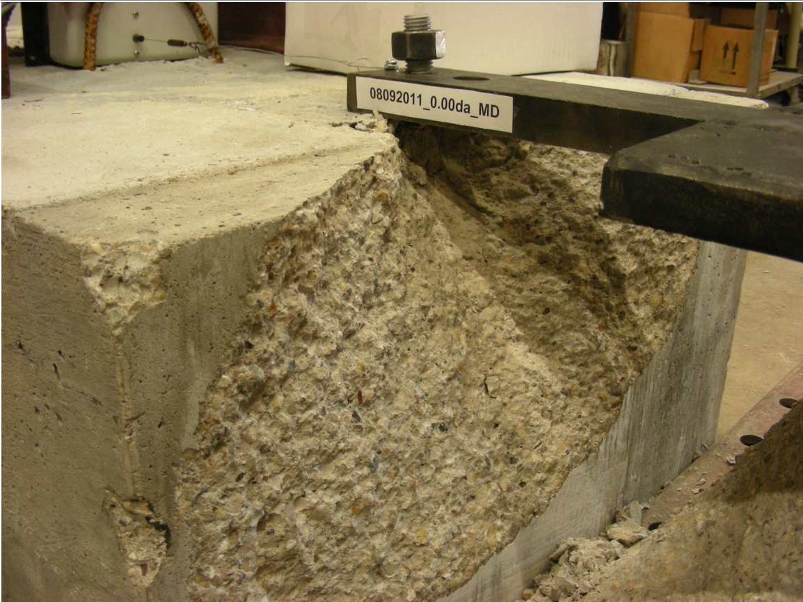
Figure I.9 Behavior of Specimen 08092011_0.00da-MD
