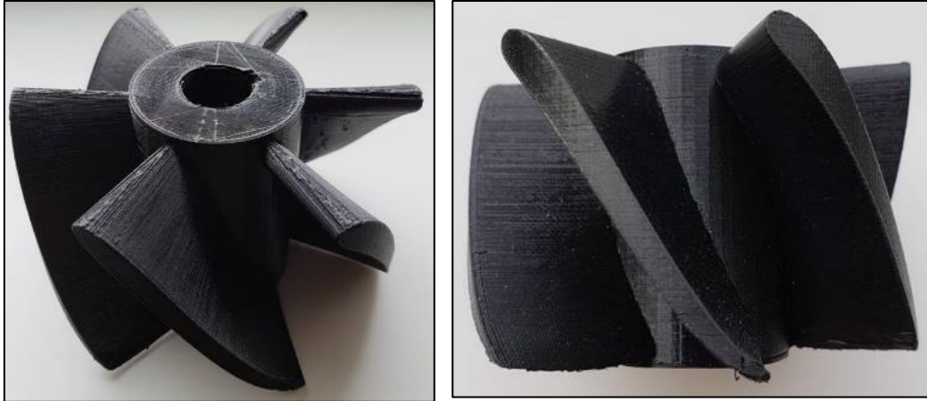
Figure 3-10: The 3D printed 7.6 cm (3-inch) 6-blade rotor for the experimental testing
