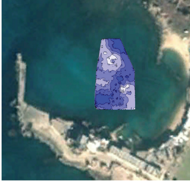
Figure 8c: Bathymetric data collected from the survey area delineated in FIG. 8a.
