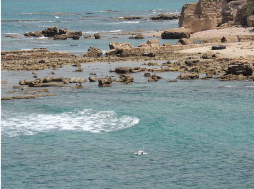
Figure 2: The Pladypos following a preprogrammed survey pattern in the intermediate Herodian harbor at Caesarea in 2014; the vehicle's ability to stay on course is not significantly affected by the 0.5 m swell.
