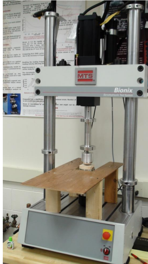
Figure 6. Compression testing machine used for the material parameters experiment
