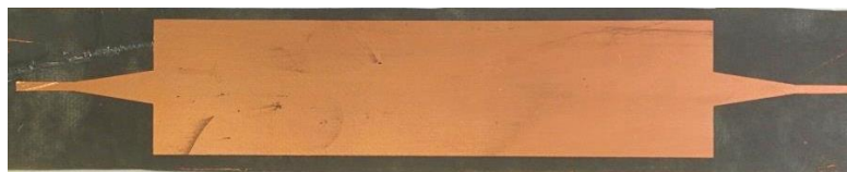
Fig 34. Photograph of the Rogers substrate with patterned top metal layer
