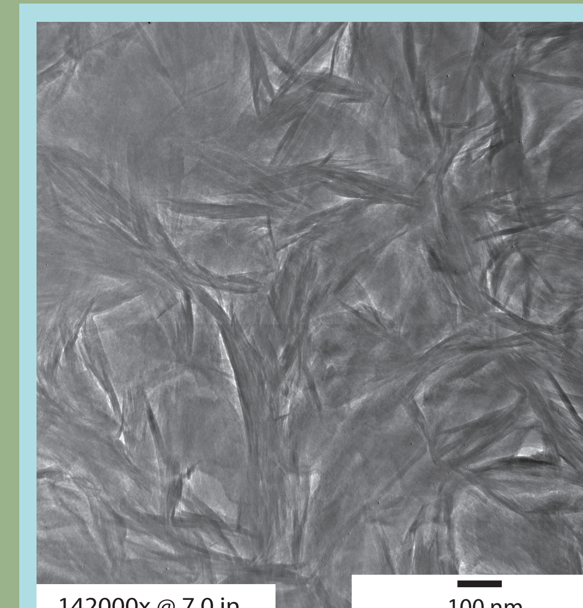
Figure 2. Illite laths in an ion milled sample.
