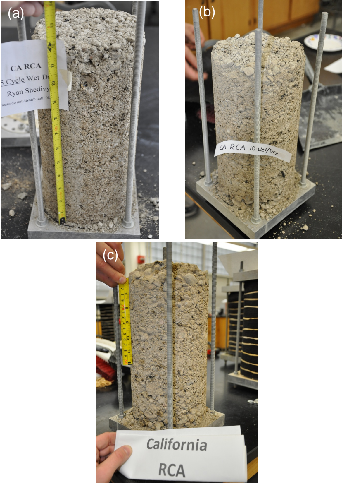
Figure 1.28 CA RCA after Wet/Dry Cycles: (a) 5 Cycles; (b) 10 Cycles; (c) 30 Cycles
