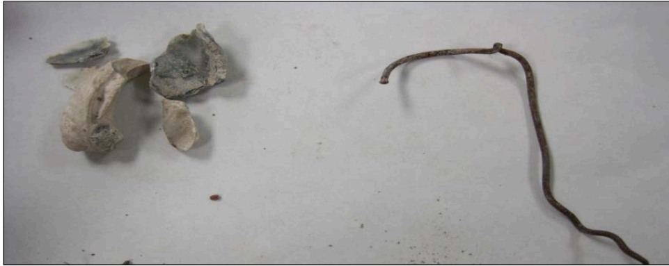
Figure A.11 Deleterious Material found in RCA: Sea Shells and Steel (Bozyurt 2011)
