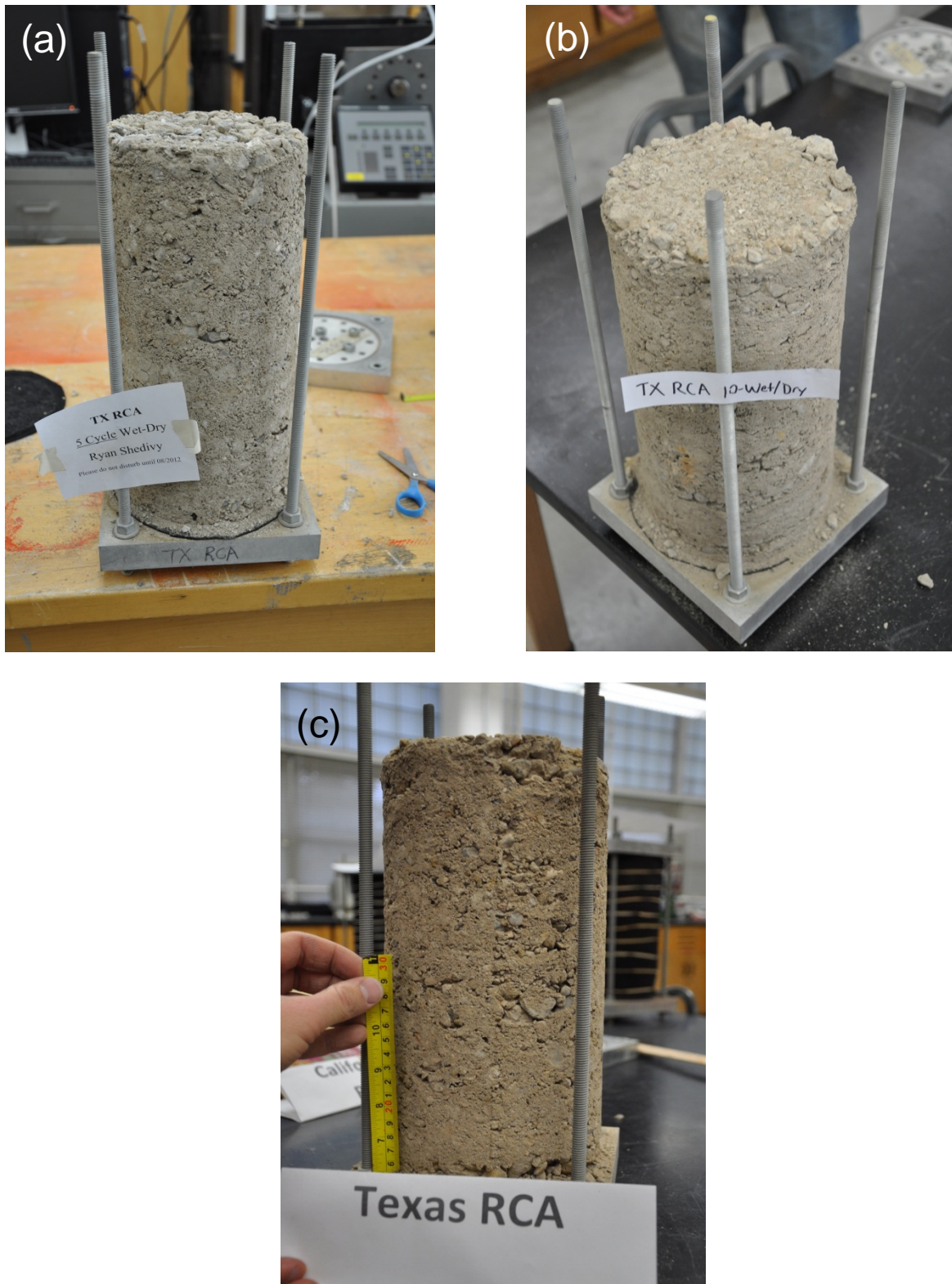
Figure 1.29 TX RCA after Wet/Dry Cycles: (a) 5 Cycles; (b) 10 Cycles; (c) 30 Cycles
