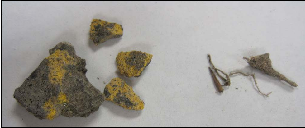
Figure A.13 Deleterious Material found in RAP: Pavement Markings and Wood Chips (Bozyurt 2011)
