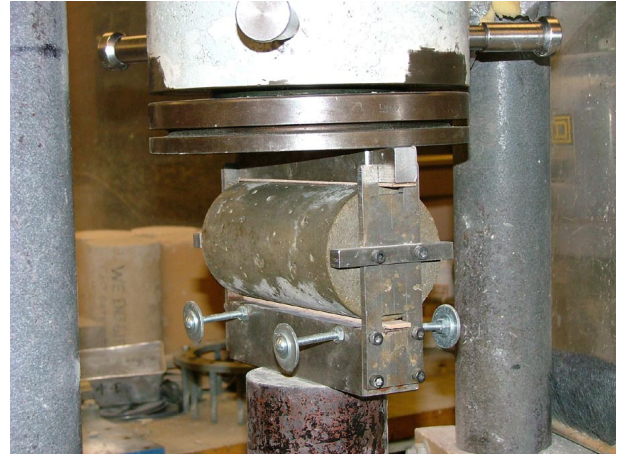
Fig. 4-2. Splitting tensile strength test of concrete
