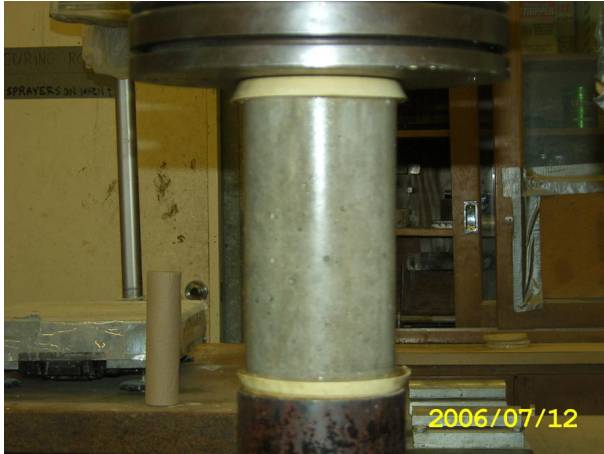
Fig. 4-1. Compressive strength test of concrete
