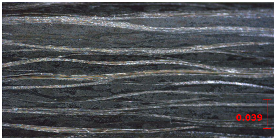
Figure 45. Optical microscopic cross-section image for CF/PEI co-mingled specimen.
