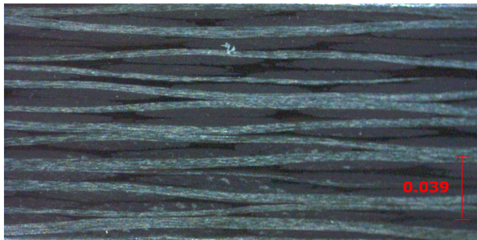
Figure 44. Optical microscopic cross-section image for CF/PEI film specimen.
