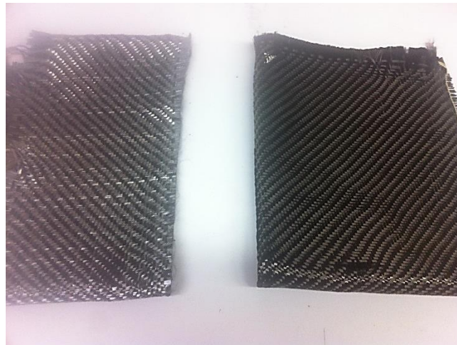
Figure 6. Co-mingled CF/PEI weave (left) and a plain carbon-fiber weave (right).
