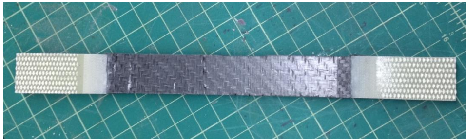
Figure 23. CF/PEI tabbed tensile sample with tapered ends.
