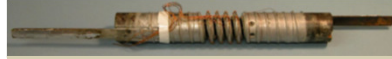
Cu-Be spring apparatus utilized for the electromechanical testing on Bi-2212 wires at UC-Boulder.
