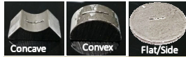
The post-testing examination of the wires: Concave shows the inner radius of the tested spiral, Convex shows the outer radius, and Flat shows the side of the wire.
