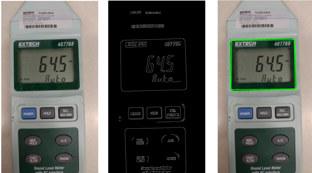
(a) Example test image (b) Canny edged feature (c) First bounding box
