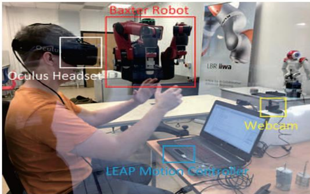
Figure 2-3 MR-based interface for human-robot interaction setup [45]
