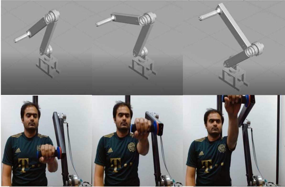
Figure 7-10: Monitoring shoulder joint flexion-extension exercise using Vuforia Studio AR platform and observing participant's upper-limb movement through Microsoft Teams video session.
