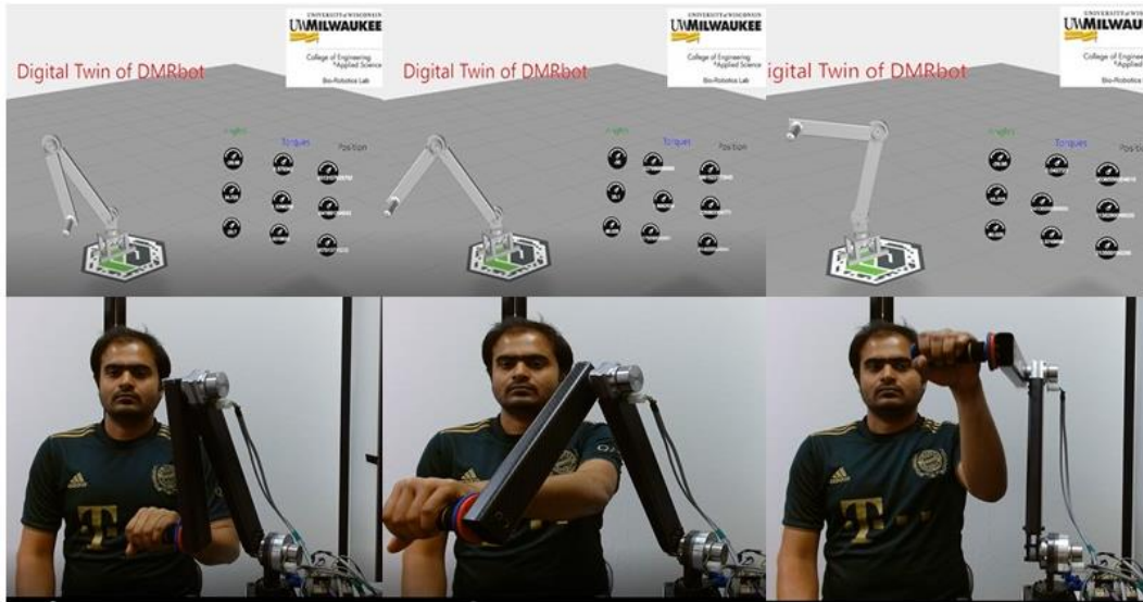
Figure 7-21: Monitoring RT control mode using a joystick to provide PRE through Vuforia Studio AR platform and observe end-effector position and participant's upper-limb movement through Microsoft Teams video session.
