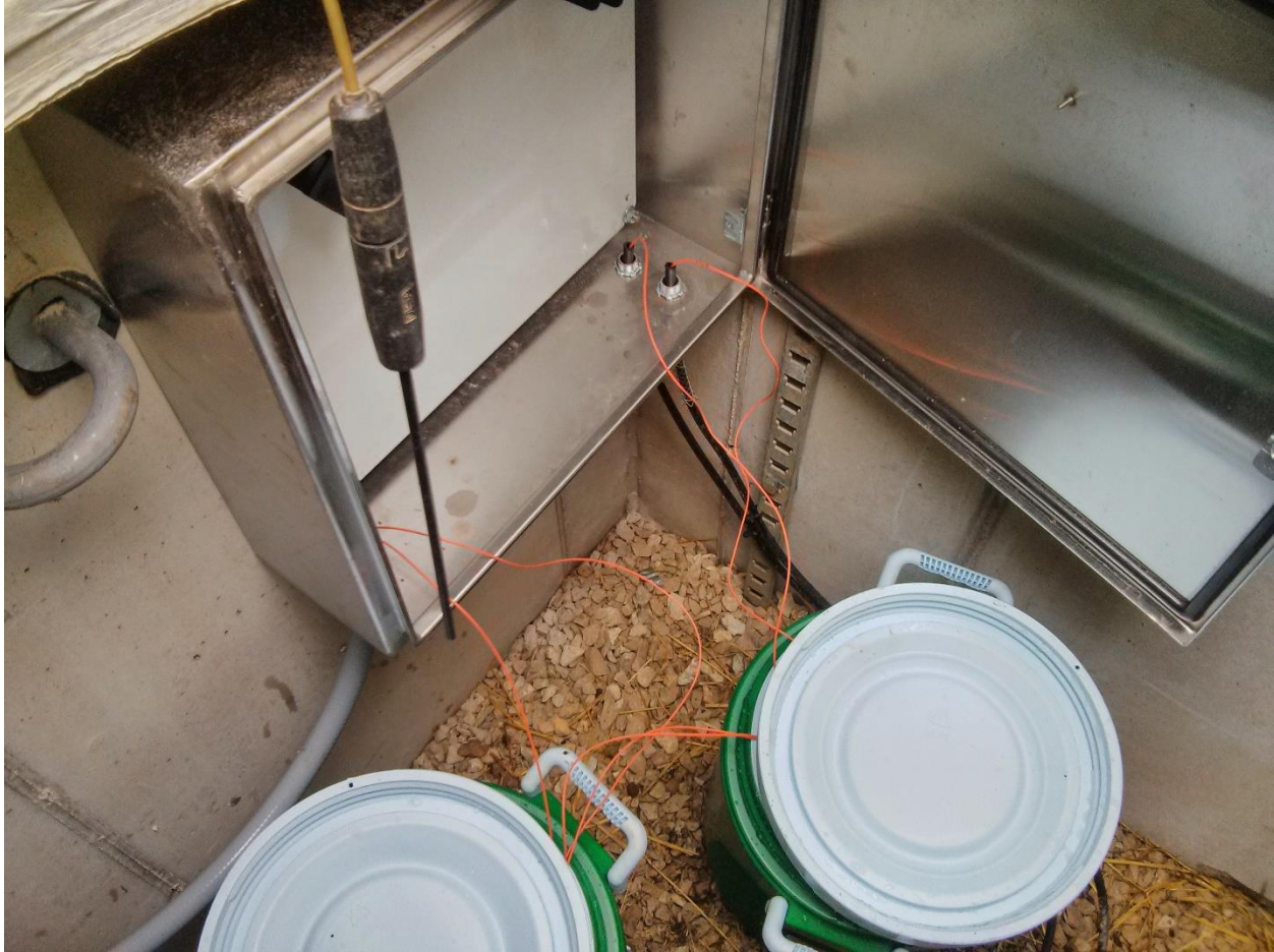
Figure 40: A photo representing a pair of calibration baths at Borefield #4. This particular pair is located in TMW-1B.
