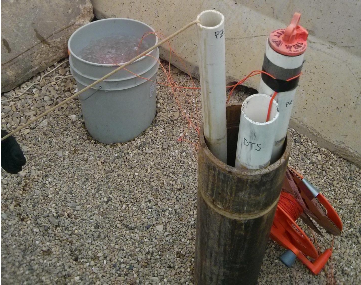
Figure 28: Easternmost piezometer nest during a temporary DTS test of the blank, which is labeled “DTS” in the photo.
