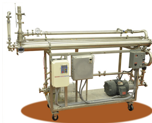
Ultrafiltration (spiral element) system
