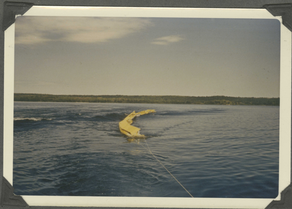
Figure 11. Towing pontoons to station and testing riding capabilities with 18 inch waves.
