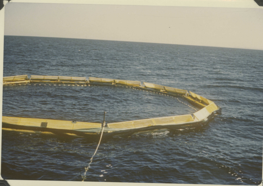
Figure 14. EDN loaded on pontoons just prior to dropping in 54 feet. Note circle of gill net floats on inside of pontoons. As before the entire 30 ft. of side curtain and lower canvas is in each trough.
