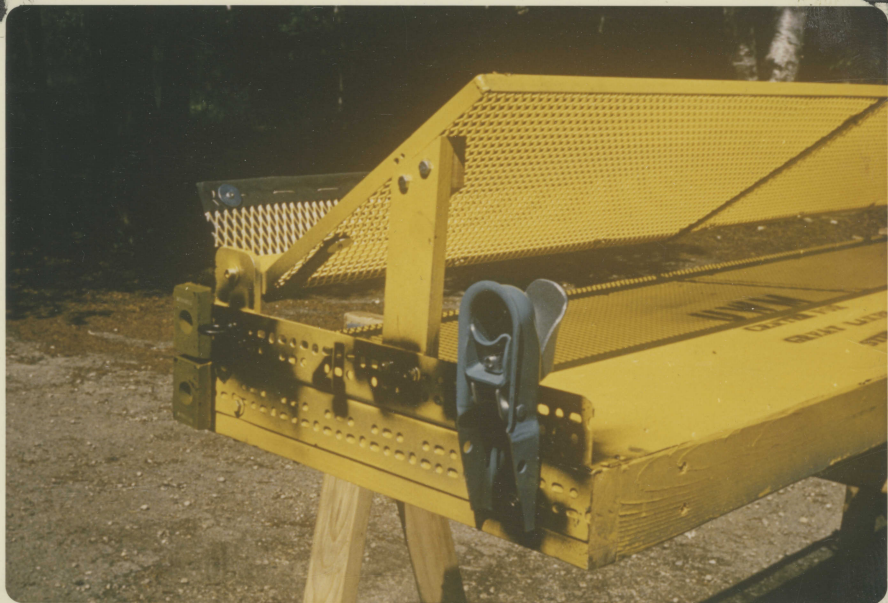
Figure 10. Modified pontoon end. Fulcrum for trough later moved to very edge of pontoon. Note rubber bumpers.
