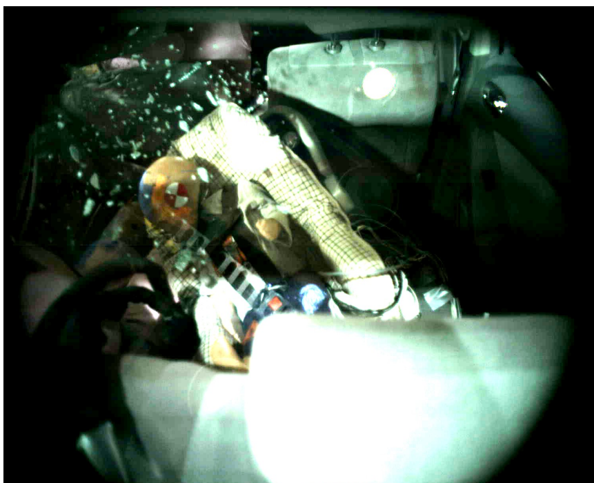
Photo 17 (NHTSA, 2007a, from high speed video) Infant carrier, 2008 Nissan Altima NHTSA SINCAP test
