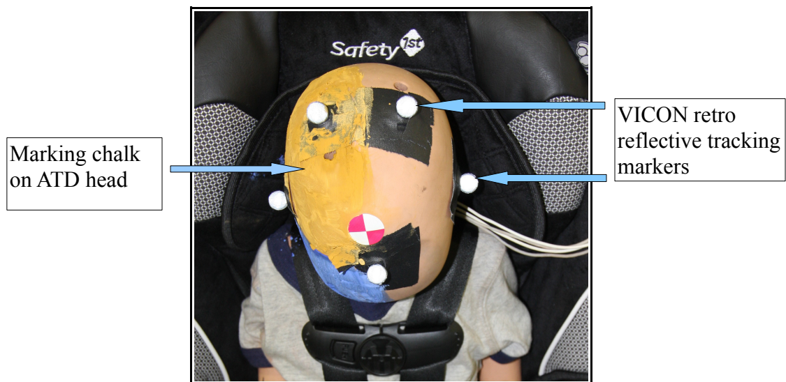
Photo 6 CRABI 12 head with tracking markers, and marking chalk.
