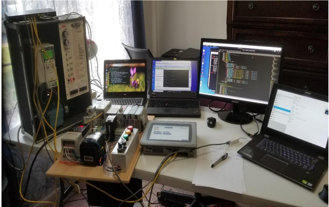
Figure 5-4. ICS testbed, including PLC, HMI, ABB drive, laptops including Kali VM
