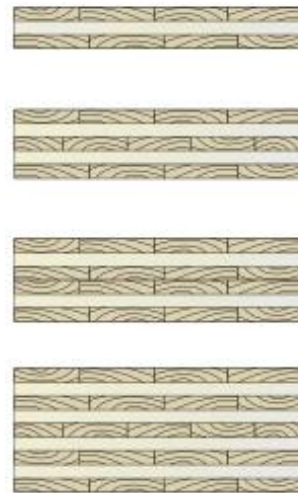
Figure 2. Sections of Common CLT Layups
