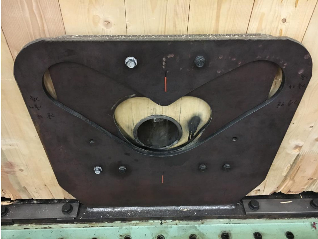
Figure 96. Wear of slotted shim edge for e = 0.88 panel in No-Slip Traction Rolling
