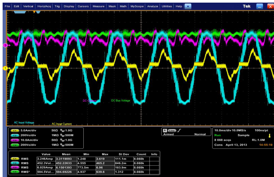
Figure 4.21: Experimental Unbalanced With DC Filters Vab, Ib, DC Bus Voltage and Current
