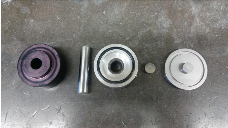
Figure 10: Die used to create pellets, disassembled. The inner diameter of the chamber was 0.500”
