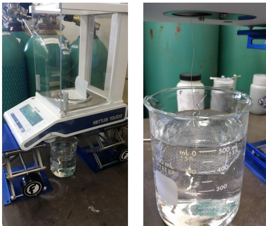
Figure 12: (Left) Scale setup used to make weight measurements for porosity (Right) Basket used to suspend pellets in second weight measurement
