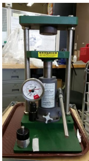
Figure 9: Press used to create pellets for sintering
