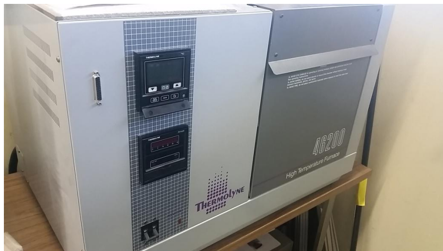
Figure 11: Furnace used to sinter pellets
