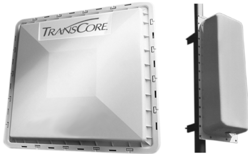
Figure 9 An Example of Toll Tag Reader and Antenna (Cited from TransCore (23))
