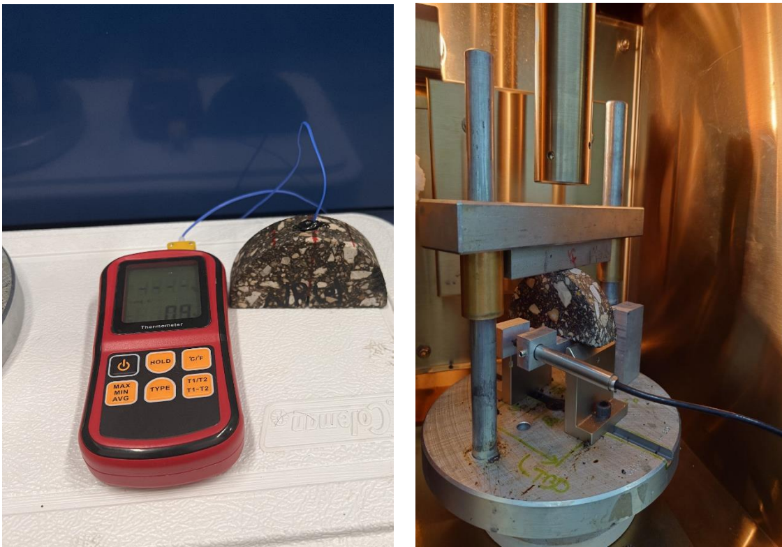
Figure 3-1: Probe used to monitor the temperature of the samples and test specimen in the MTS frame.
