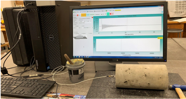
(a) Longitudinal resonant frequency test of PCC cylinder
