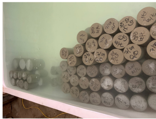
Figure 3.5: Picture of the various steps taken to prepare PCC test cylinders.
