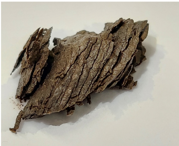
(a) shale from dolomitic limestone aggregate sample
