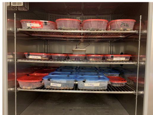
Figure 3.4: Freeze-thaw test system used to process the investigated coarse aggregates
