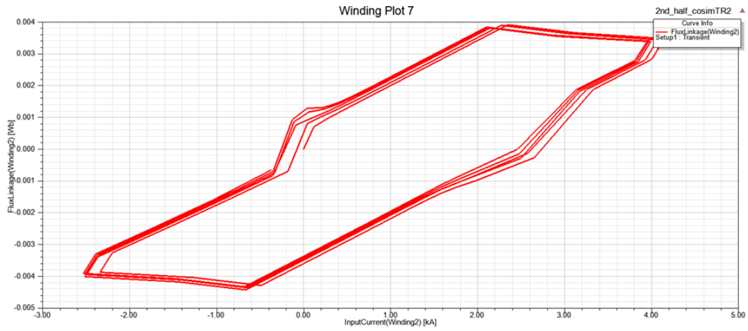
Figure 2.54. Flux linkage-input current for winding 2 (2400V).
