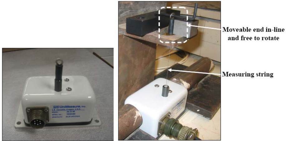
Figure 4.3 String potentiometer (draw wire transducer – DWT) used in this project.
