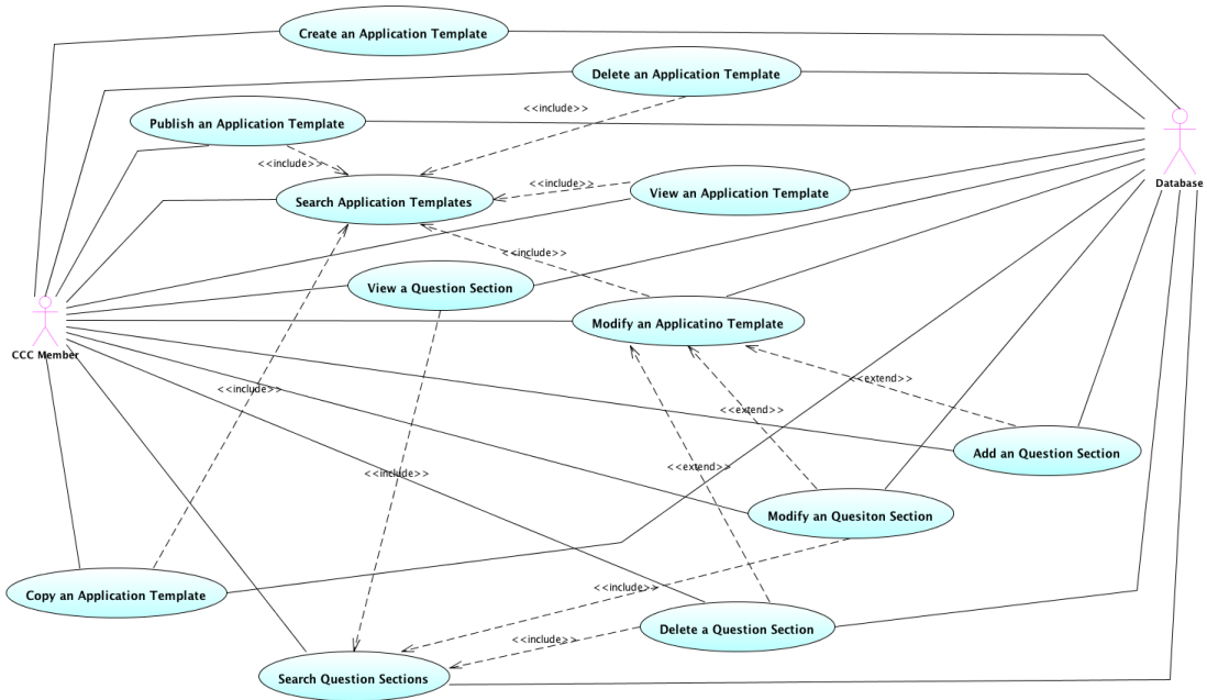
Figure 34. Use Case Diagram for CCC Member Application Template Management
