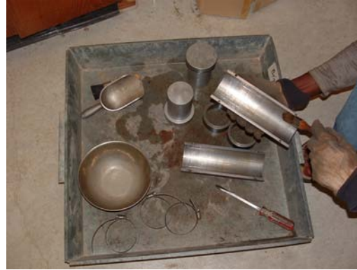
(b) Lubricating the mold
