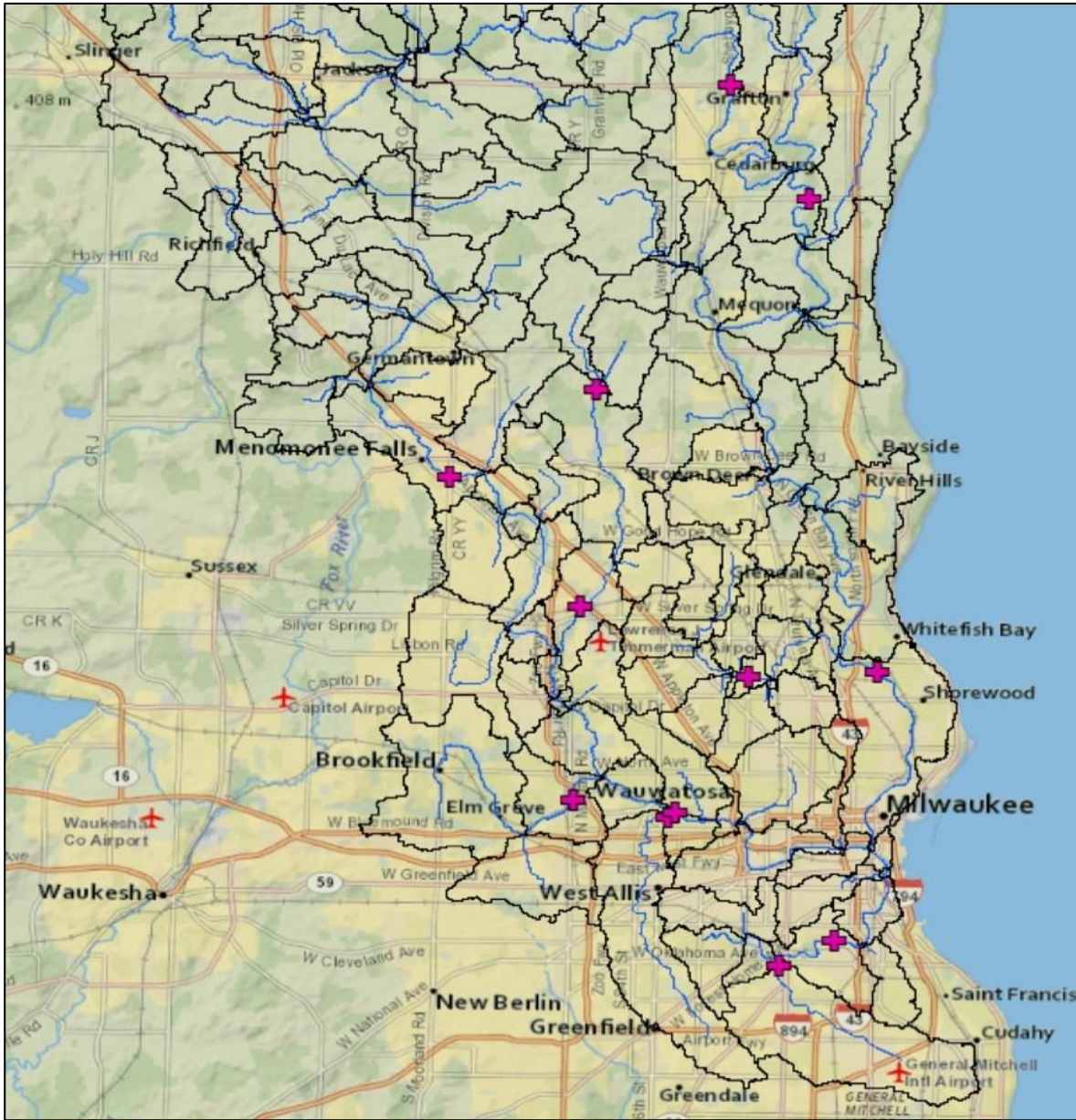
Figure 2.5 Locations of USGS stream gage stations where stream flow rate data were extracted for HEC-HMS model calibration
