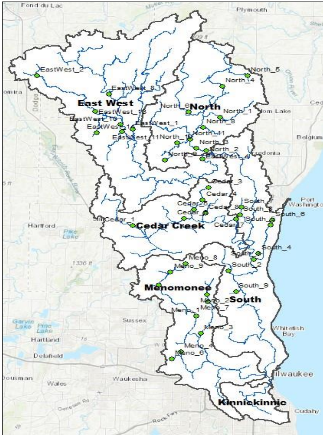
Figure 3.2 Distribution of beaver dams identified for hydrologic modeling. Solid circles indicate dam locations and blue lines represent the stream network in the HEC-HMS model
