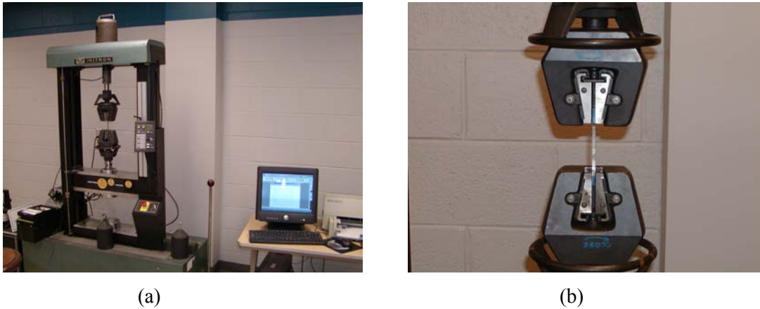
Figure 2.22: Tensile Testing Machine and Fixturing Used for Material Characterization Study.
