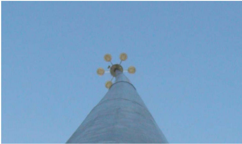
Figure 3.78: Displaced Shape of HML-67-006 During 20-30 mph Peak Gusts.
