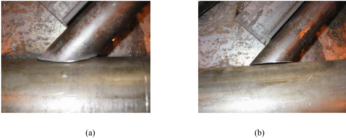
Figure 2.20: Saddle Connectivity: (a) Back-ground or Fish-Mouth Specimen; (b) Non-Back-Ground or Straight-Cut Specimen (Peronto 2003).
