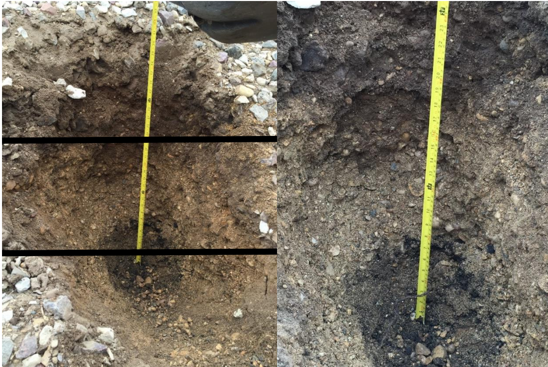
Figure 37: Test pit pictures from different angles. Picture on the left has rough delineation of soil layers
