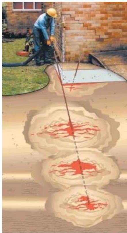
Figure 3: URETEK Injection System ( www.uretek.com )
