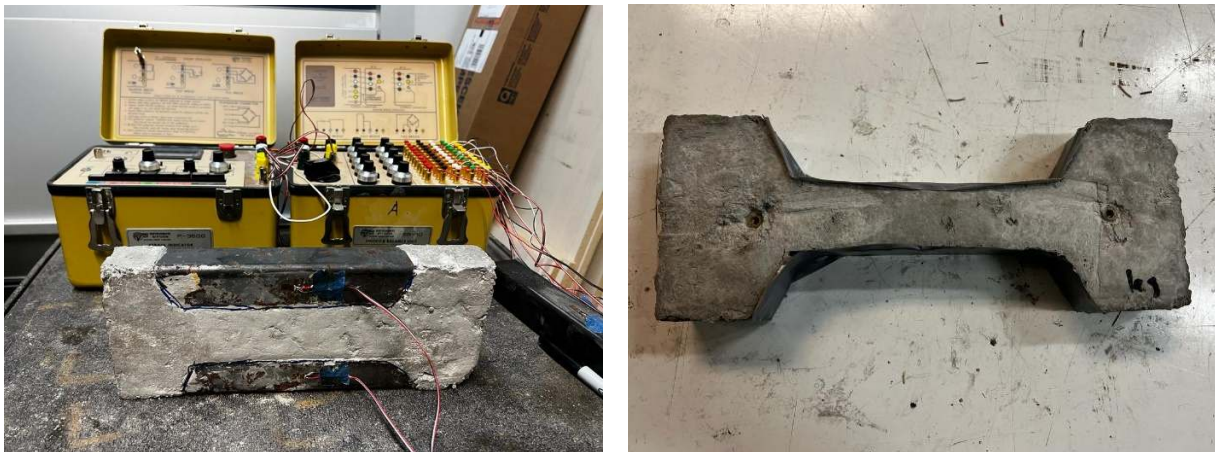
Figure 7 Restrained and Unrestrained dog bone specimens
