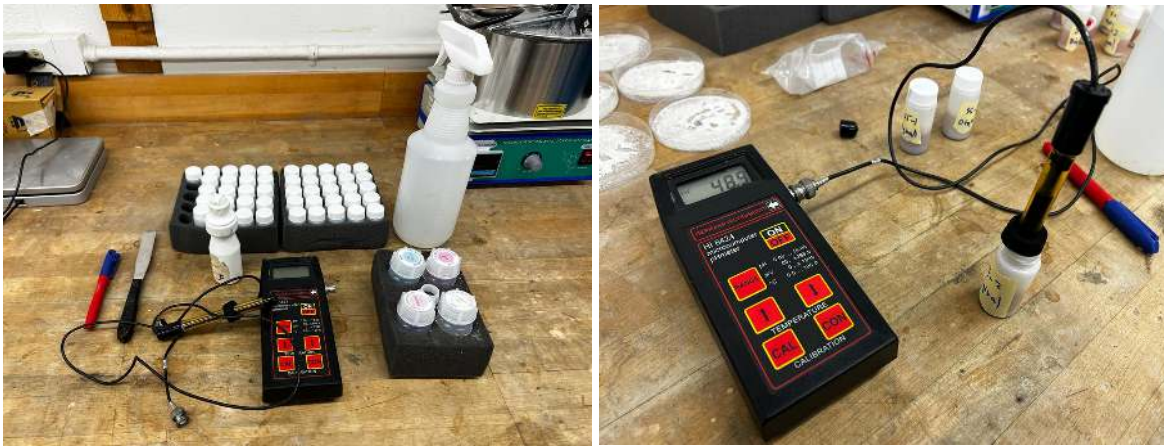
Figure 11 Rapid Chloride test setup and measurement
