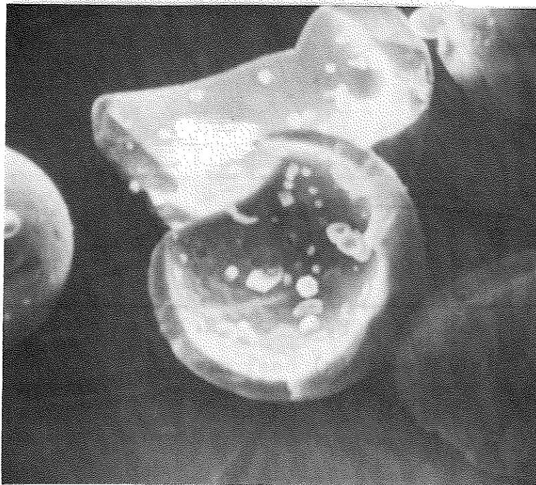
Figure 11. Partially Broken Particle from Benzyl Alcohol Emulsion with Low Solids Content (500x)
