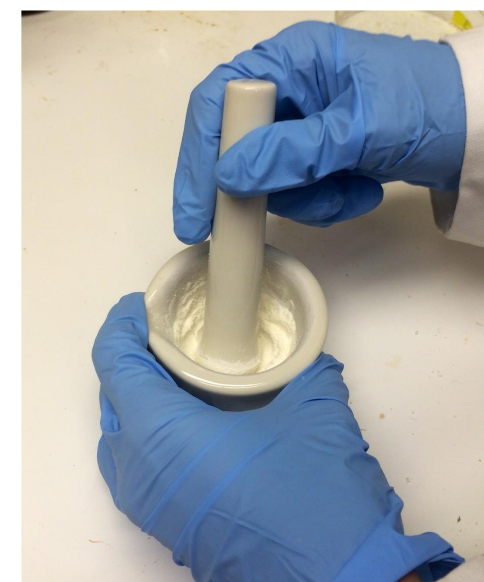
Manually encapsulate AITC in TA \beta CD (left) Encapsulating AITC in TA \beta CD by stirring (right)
