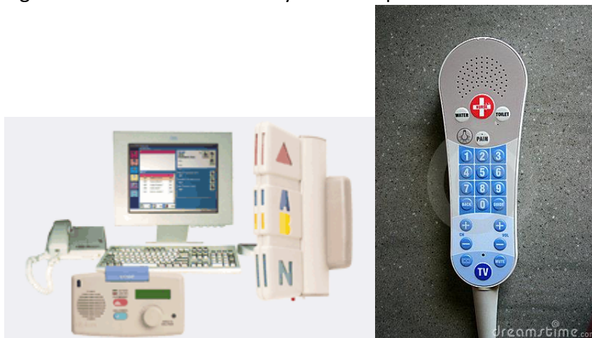
Figure 1. Hill-Rom Nurse Call System Components
