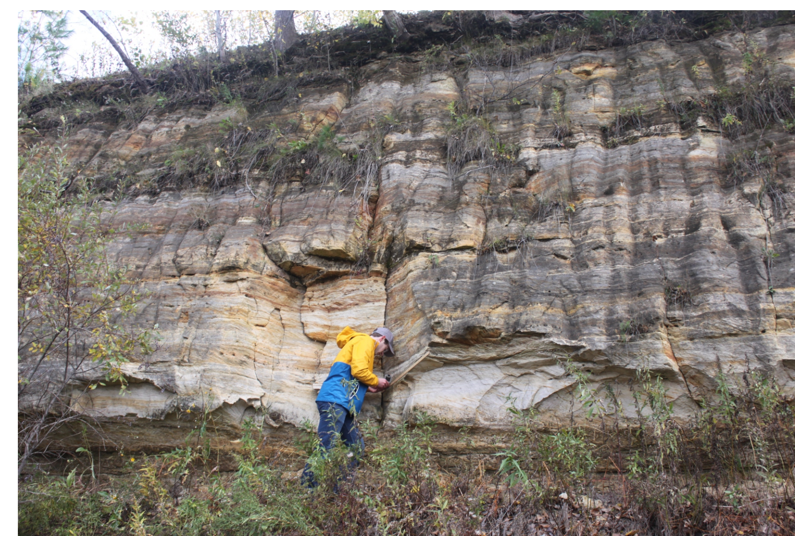
Fig 10. Outcrop measurements where fracture orientation were obtained along Wisconsin State Hwy 37 immediately below Huntsinger Heights subdivision.
