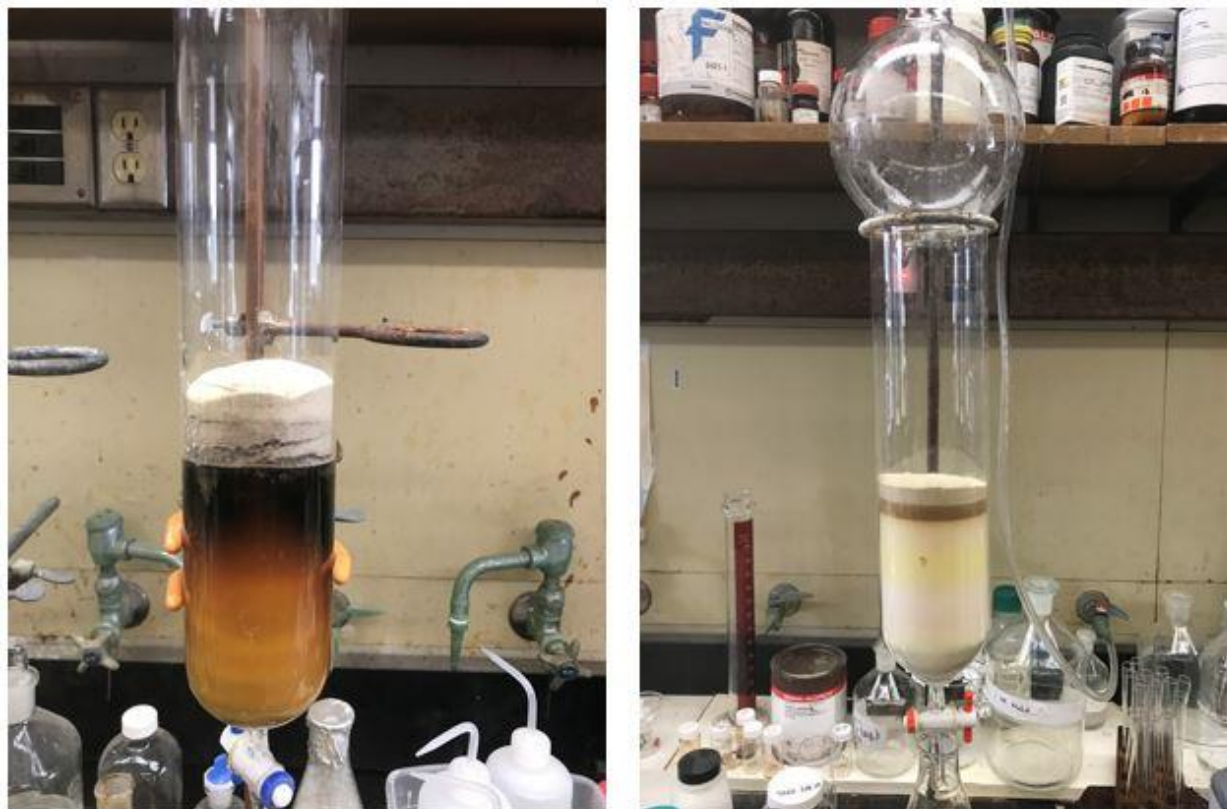
Figure 100. Effect of removal of \text{ZnCl}_2 from the reaction mixture in the second step of the synthesis of 2'- \text{CH}_3 5-bromo 2-bminobenzophenone 68. Left image shows the hard mass formation due to the solidification of \text{ZnCl}_2 after wet loading in column chromatography. Right picture shows the effect of complete removal of \text{ZnCl}_2 from the reaction mixture.
