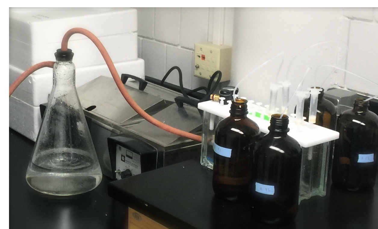
Fig. 4: PPCP extraction apparatus: pump, waste container, vacuum manifold, SPE cartridges, fritted glass filter with tubing
