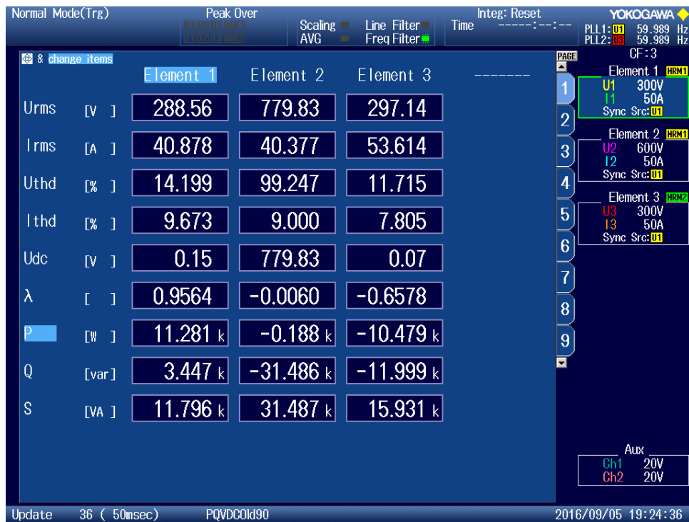
Figure 120 - Measurements of "PQ" Supplying -0.57 pu Active and -0.57 pu Reactive Power at 4500Hz
