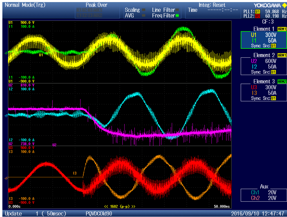
Figure 123 - "PQ" Supplying -0.8 pu Active Power Step at 4500Hz (50ms Window)
