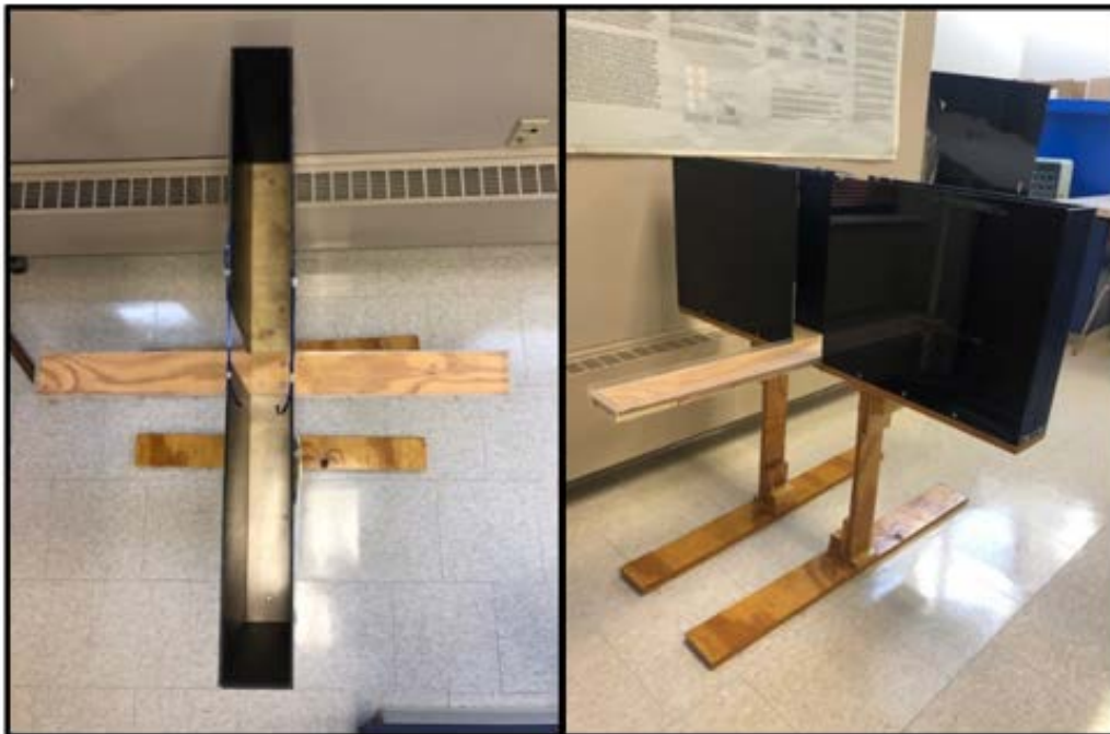
Figure 3. Elevated plus maze. The elevated plus maze has two open arms, two closed arms, and is raised 21.5" off the ground.
