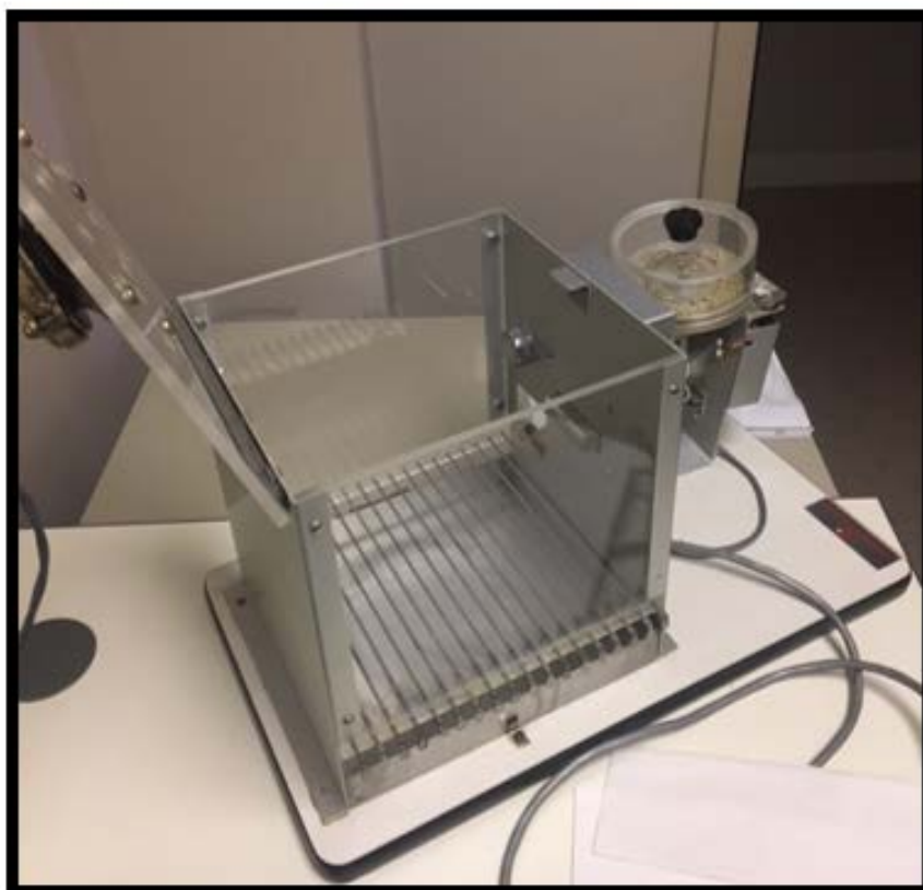
Figure 1. Operant chamber. The recessed food cup is positioned in the bottom left of the cage. The lever is centrally located, and the illumination light is directly above the food cup.
