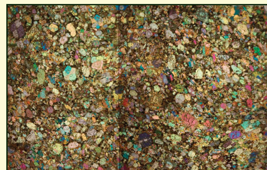
Figure 3. Photograph of polarized thin-section from Haystack Butte at 20x magnification.
