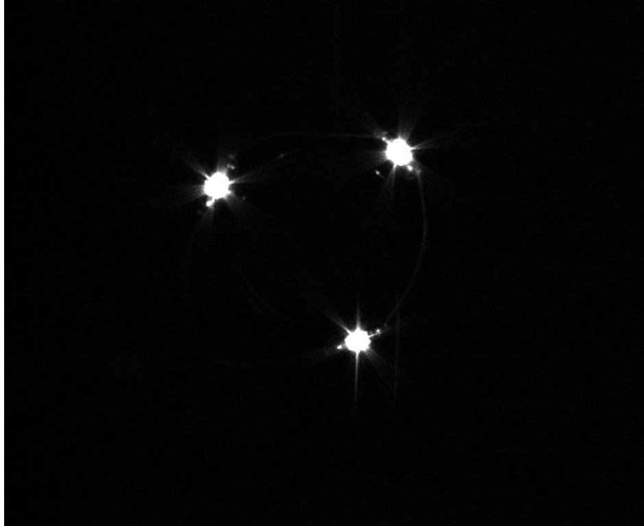
Figure 4-10 Example of an image taken by the Allied Technologies camera; this image is processed through an algorithm to triangulate the center of the mirror.
