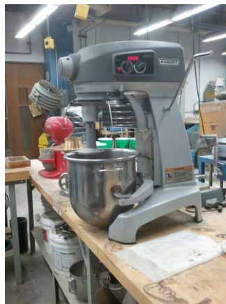
Figure 11 Mixing of PVA-ECC using Hobart mixer
