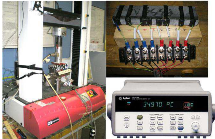
Figure 20 Experimental setup for 4 point bending and electrical measurements
