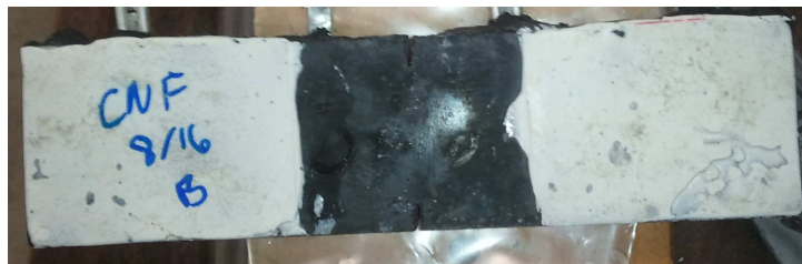
Figure 23 Epoxy coated zones of samples
