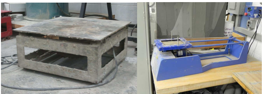
Figure 13 Vibrating table (left) and Jolting table (right) used for compaction of ECC
