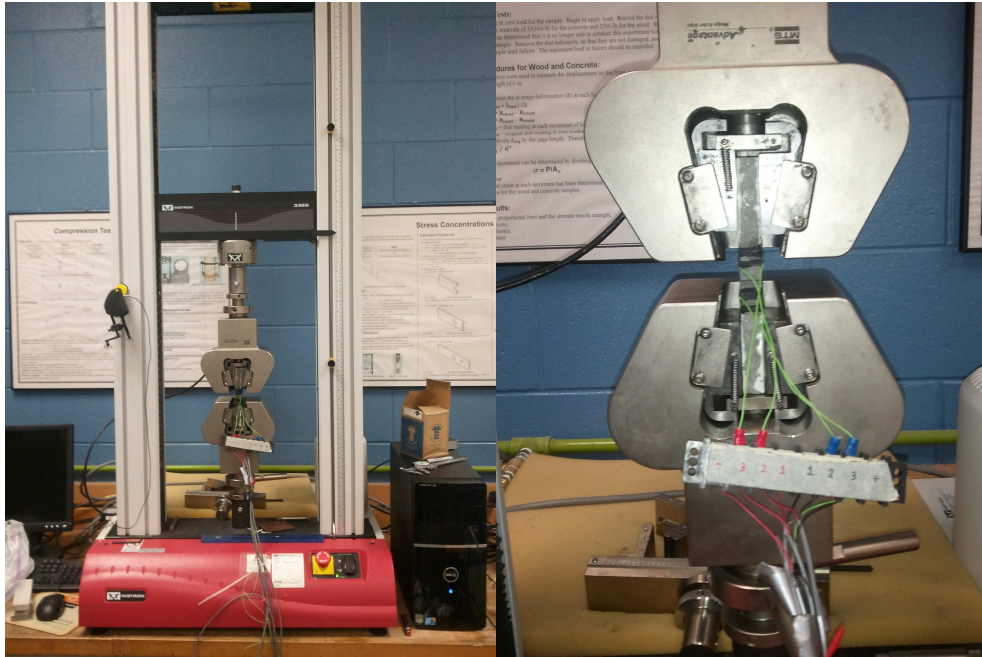
Figure 22 Experimental setup for tensile testing
