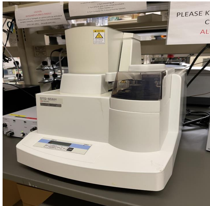
Figure 11: DTG-60AH From Shimadzu in The Global Water Center UWM
