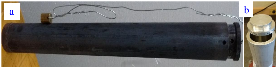
Figure 42: Crucibles that was used to melt Mg (a) low carbon steel permanent crucible(b) Mg sacrificial crucible.
