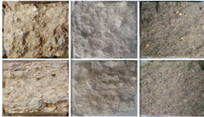
(a) Gravel-cement (b) Gravel-fly ash (c) Sand-cement
