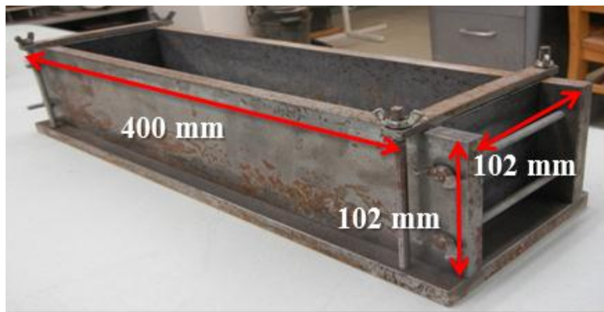
Figure 3.10 Prismatic Beam Molds
