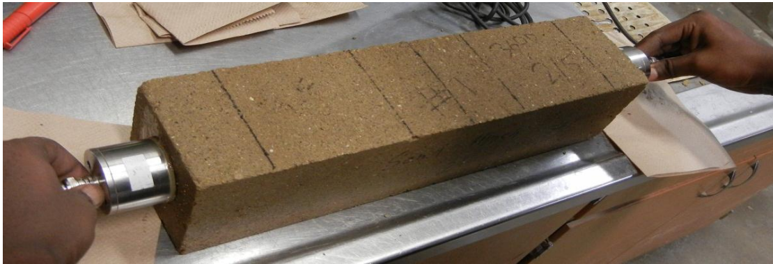
(a) Testing on beam specimen using PUNDIT-PLUS
