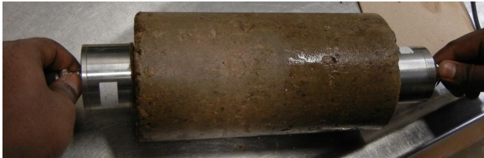
(b) Testing on cylindrical specimen using PUNDIT-PLUS
