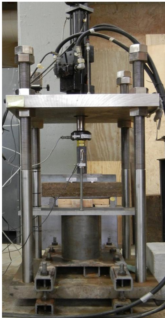
Figure 3.15 Laboratory Setup for Flexural Strength Test
