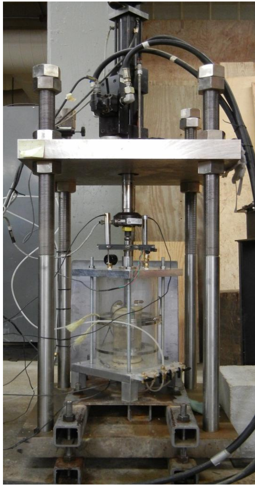
Figure 3.20 Laboratory setup for resilient modulus test
