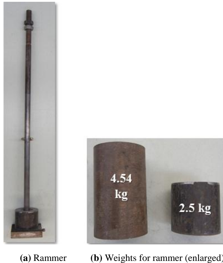
Figure 3.11 Rammer used for Compacting Beam Specimens
