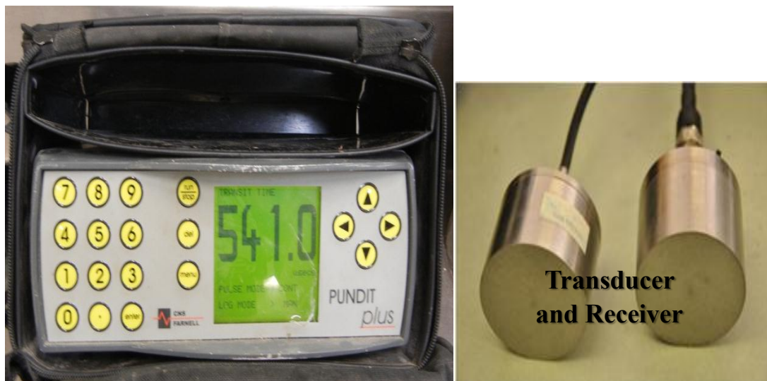
Figure 3.21 Ultrasonic pulse velocity test equipment (PUNDIT-PLUS)
