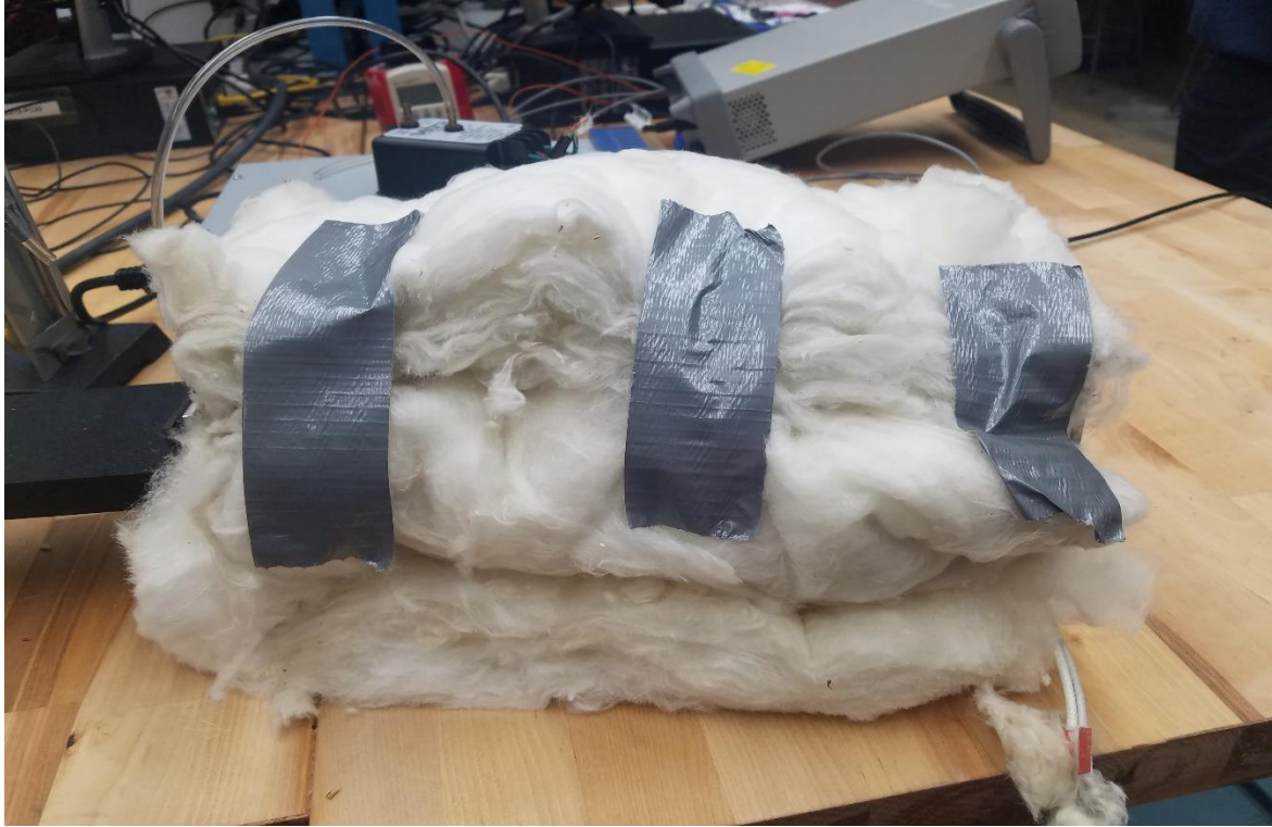
Figure 7.25 Fiberglass insulation around the fin assembly.
