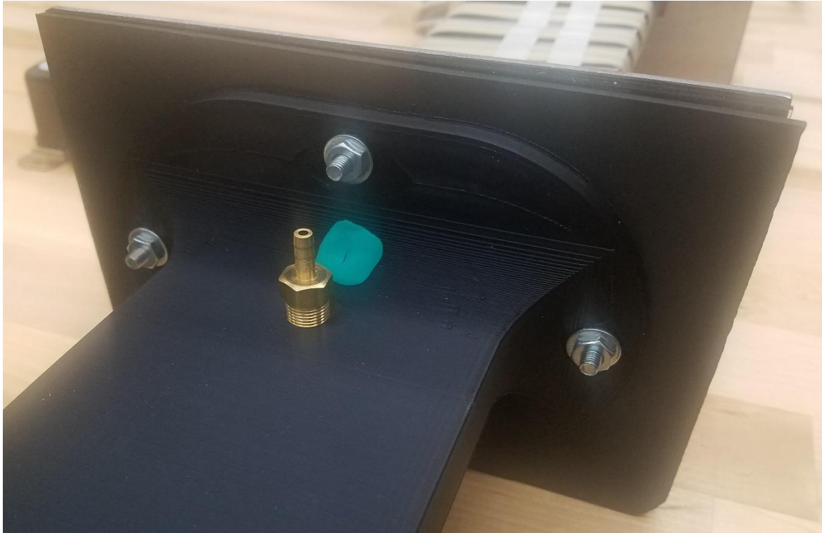
Figure 7.19 Additional fixtures to attach fin assembly and pressure gauge with the inlet channel.
