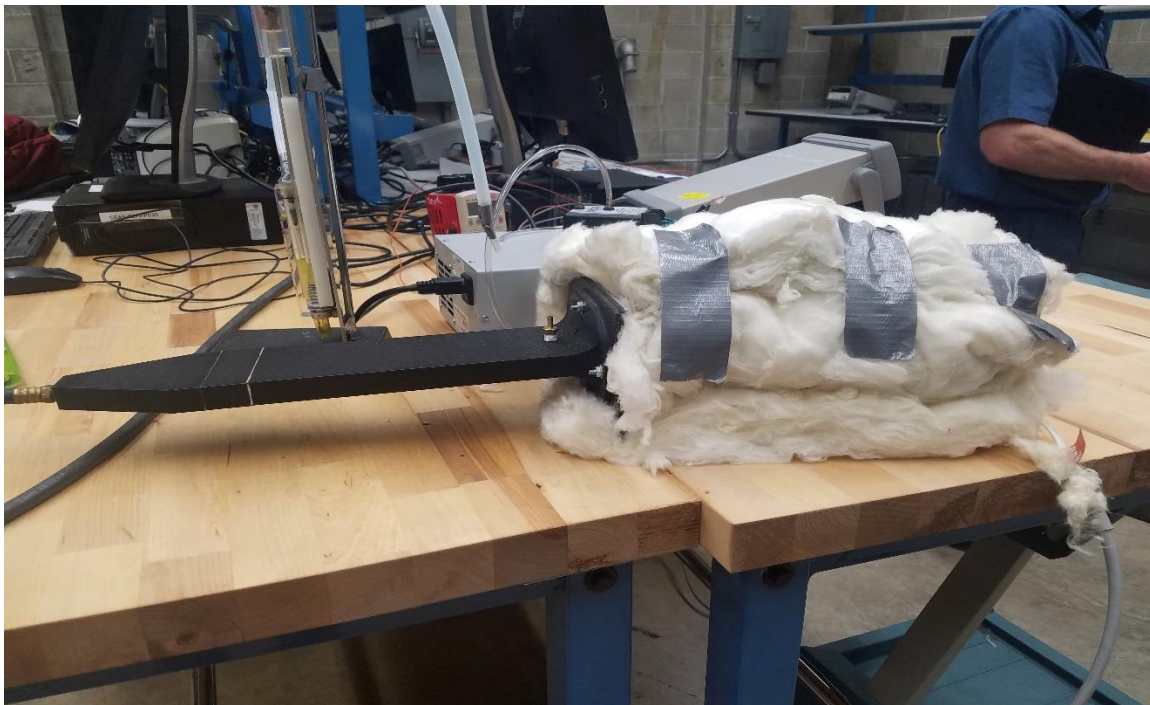
Figure 7.24 Final setup using fiberglass wool insulation.
